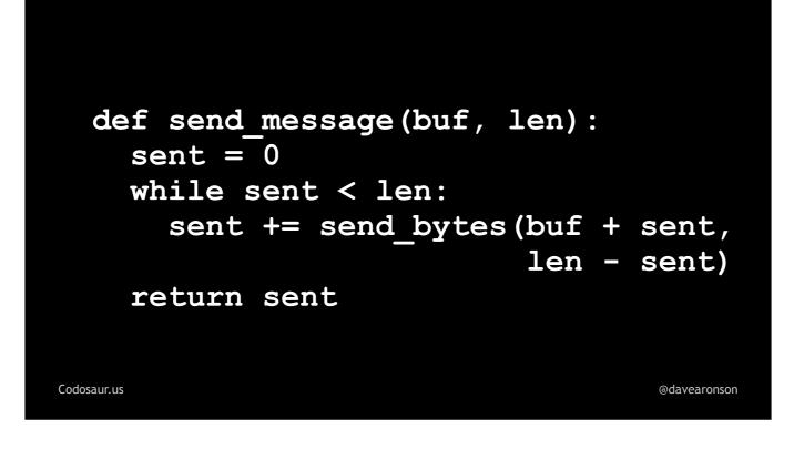
... like so. This function, send\_message, uses send\_bytes to send as many bytes as send\_bytes could send, like a woodchuck, looping to pick up where it left off, until the message is all sent. This is a very common pattern in communication software.
